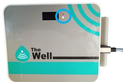
Red light indicates that the box is charging. When the box is fully charged the light will turn green.
